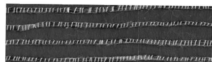
rCF-nylon-hybrid yarns scanned in reflective
