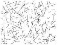
Fig. 1: Single rCF scanned at 3200 dpi
