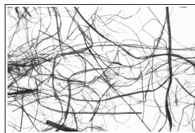
2,4 cm Hemp fiber bundles, measured with Fibreshape
