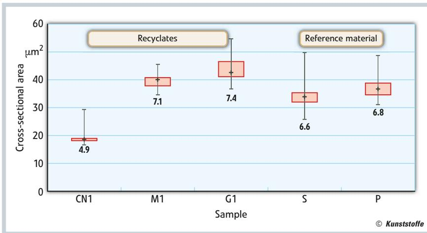
Fig. 4. Cross-sectional area distribution indicating the mean diameter (mean diameter in µm calculated from the median cross-section area via the circle formula)
