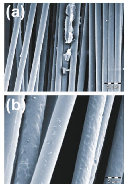
Fig. 5. (a) Matrix residues on sample M1 and (b) crater formation on sample CN1 as typical examples for irregularities
