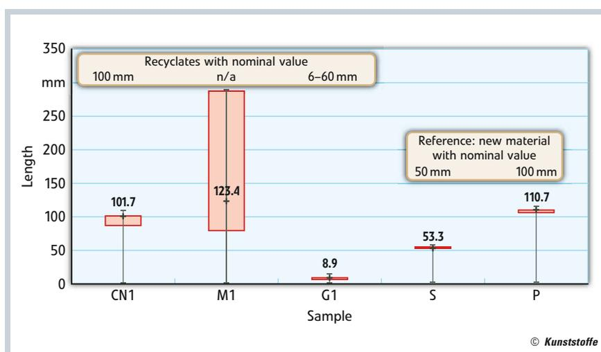
Fig. 2. Length distribution of the roving snippets with median values (n/a: not available)
